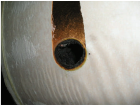
FIGURE 1: The effect of repetitive overvoltages on a transformer winding.
