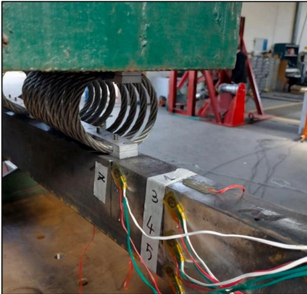
Fig. 17. Shock test with mountings: strain gauges no. 1 (top faceplate), 3, 4, 5 and 7 (web) set up.
