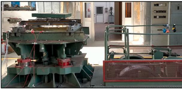
Fig. 16. Shock test with mountings: effects immediately after the drop hammer (image taken from recorded video).
