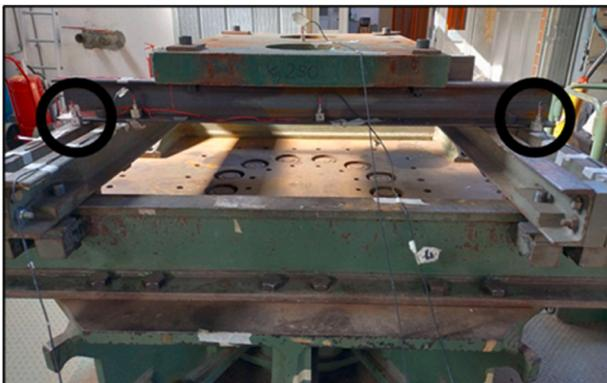
Fig. 7. Rigid shock test: accelerometers setting. Accelerometers on supporting channels are circled.
