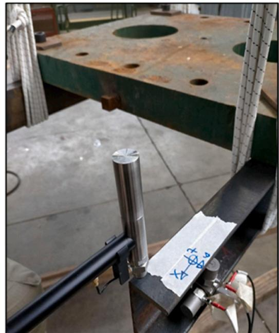
Fig. 3. Experimental modal analysis: vertical hammer and accelerometers in point no. 1.
