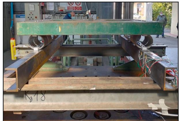
Fig. 15. Shock test with mountings set up.
