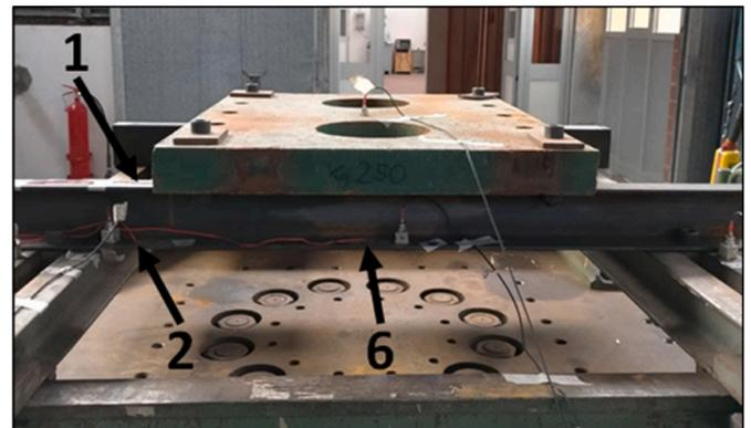
Fig. 9. Rigid shock test: strain gauges no. 1 (on top faceplate), 2 and 6 (on bottom faceplate) set up.
