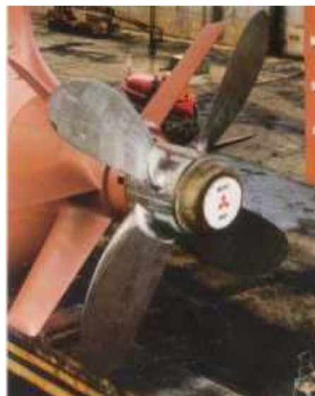
Figure 1. Pre-swirl stator ahead of the propeller cause to increase the thrust of the propeller
