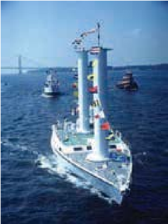
Figure 3. Flettner rotors are vertical, cylindrical sails spinning around their axis
