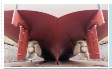
Fig. 1 Propulsion installation for a typical Ropax ferry.
