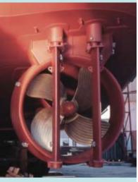
Fig. 11 Examples of propeller nozzles used by Wärtsilä.
