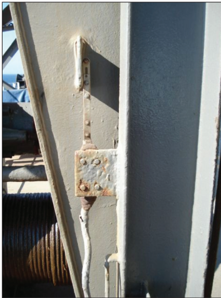
Fig. 4 Limit switch for winch motor
