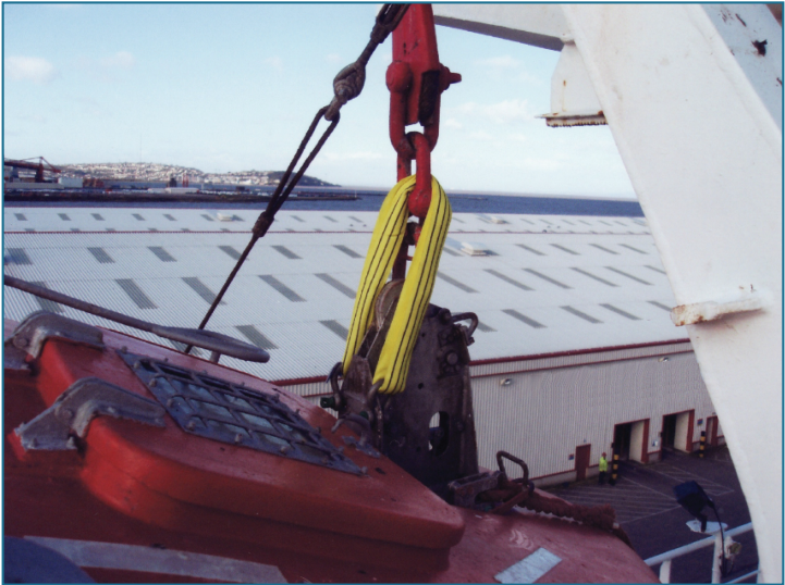
Fig. 5 A synthetic stop as a fall preventer device
