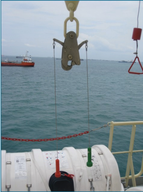
Fig. 12 Off-load release hook for davit launched liferaft
