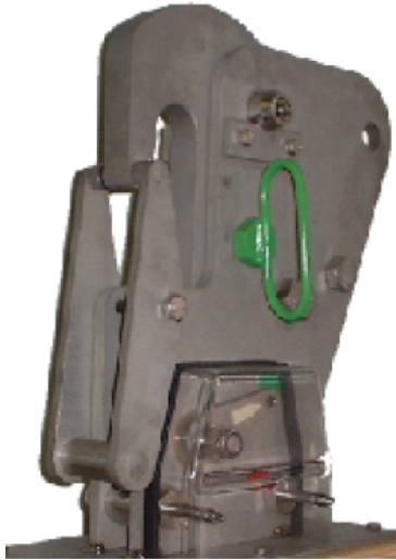
Fig. 6 A safety pin used as a fall preventer device
