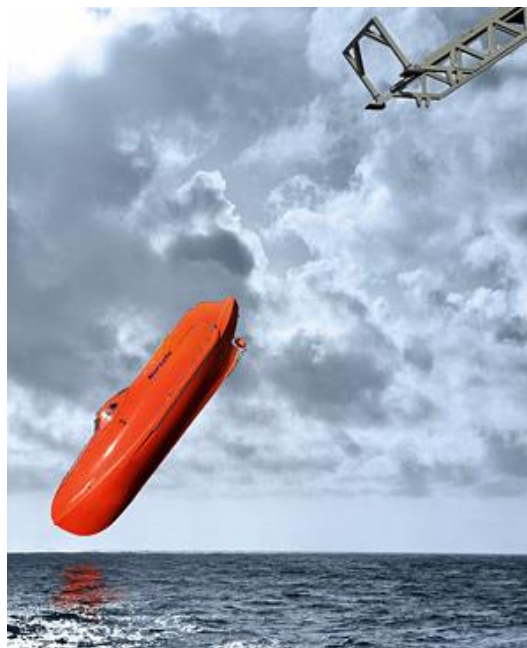
44 Figure 1: A lifeboat is about to entry water following its freefall launch (photo credit: VIKING Life- 45 Saving Equipment A/S).
