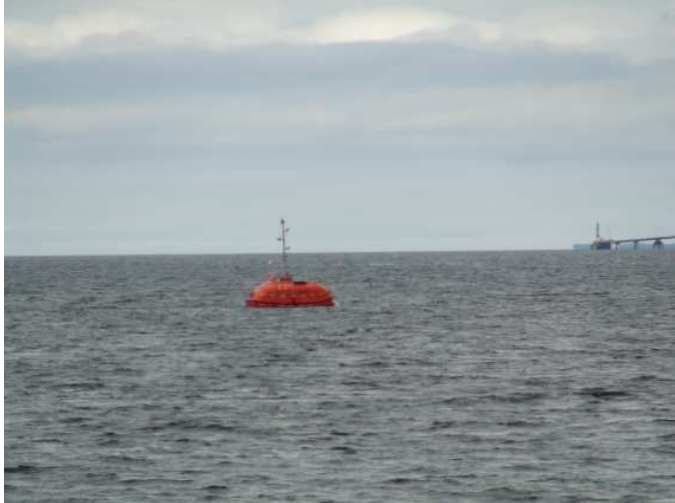
Figure 1 NRC-IOT SOLAS approved 20-person lifeboat
