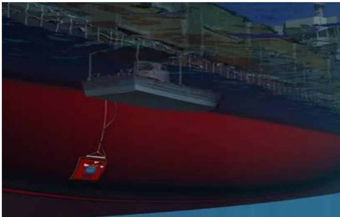
Figure 2: HST Vessel and Applicator treating a ship.
