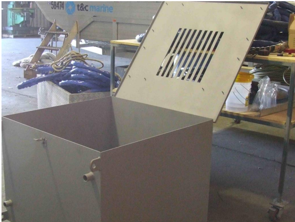
Figure 15: Sea Chest after paint with screws for settlement plates and temperature logger placement.
