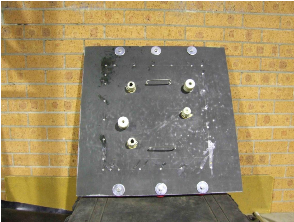
Figure 17: Replica applicator with handles, hose valves and thermo couple inlets
