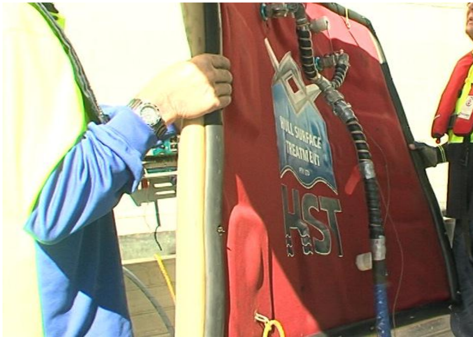
Figure 3: HST applicator with inhalant and exhalent hoses attached.
