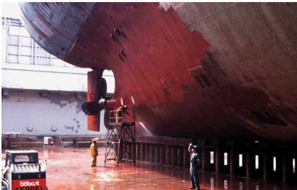
A commercial vessel in drydock undergoing hull cleaning and antifouling paint renewal.
