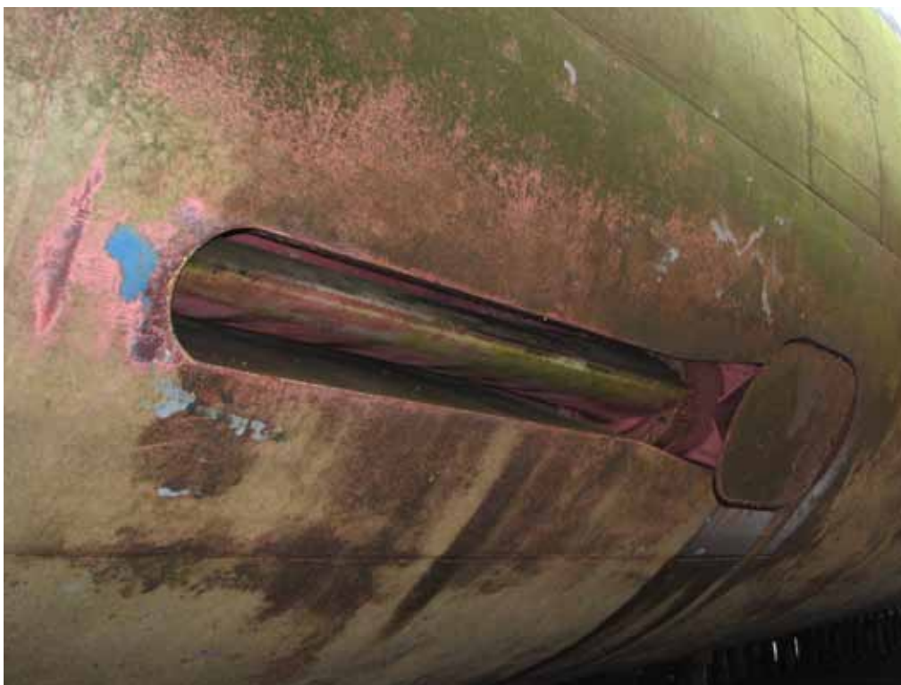
A retracted fin stabiliser with evidence of primary biofouling, a popular niche area for accumulation.
