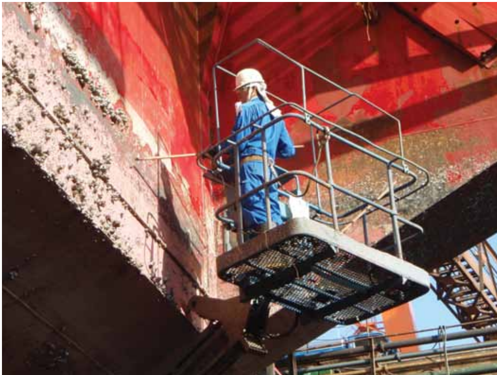
Hand scraping biofouling in drydock
