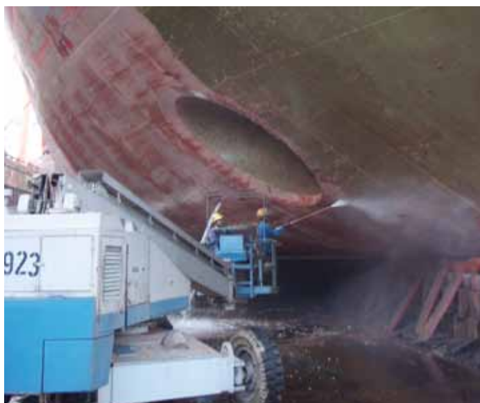
Hydroblasting biofouling from a vessel in drydock
