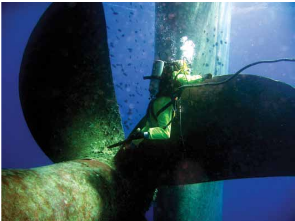
Divers checking biofouling during an in-water inspection.
