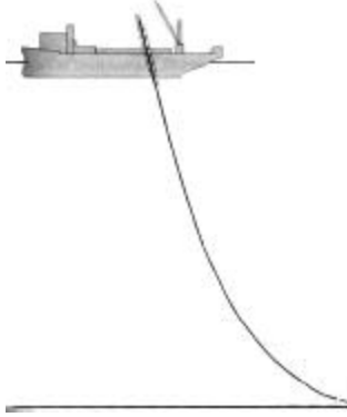
Fig.3. J-lay launching operation (adapted from Bray, 1998)
