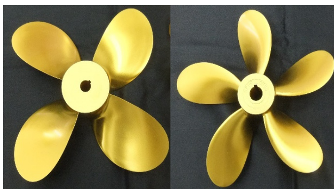
Figure 7. Photograph of model propeller. (Left: fore propeller; right: aft propeller).
