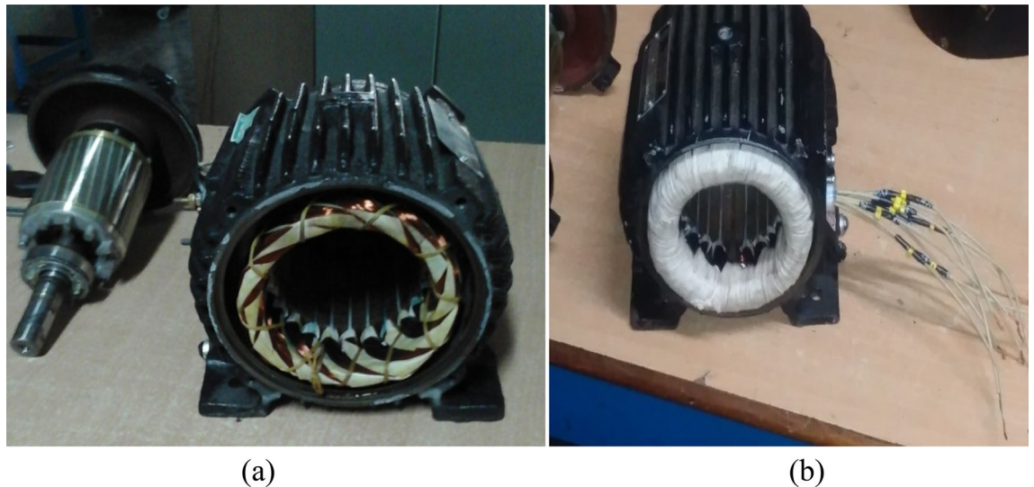
Figure 15. (a) Conventional 3 phase IM stator and rotor. (b) Proposed FPIM stator core.
