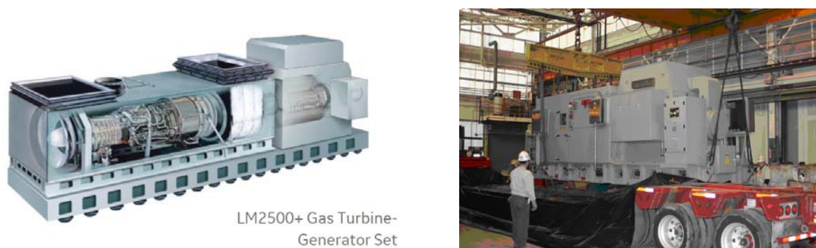
Figure 6: GE LM2500+ GTG [13] (left), GE LM500 Auxiliary GTG (right)
