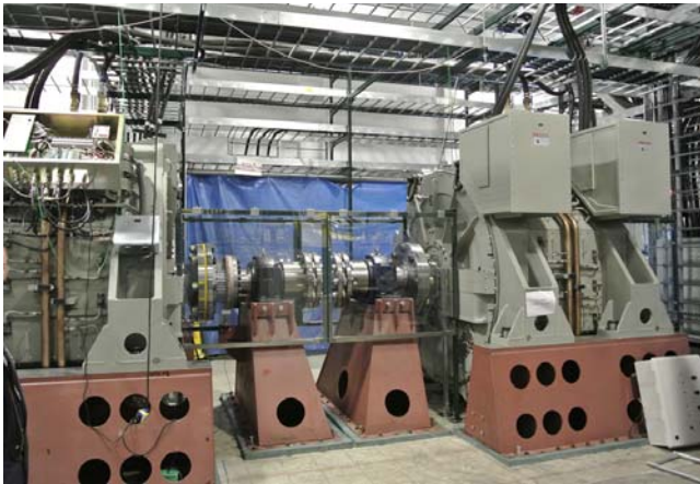
Fig. 3. Full power integration testing of the FFX-II HED system at Leonardo DRS-Naval Power Systems, Inc. (Milwaukee, WI).
