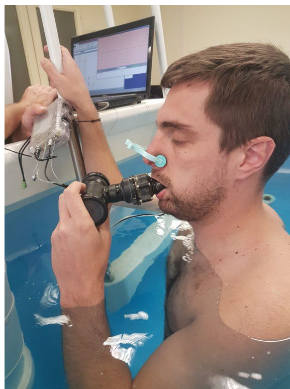
Fig. 1 A subject during measurement of immersed static respiratory compliance. The subject is kneeling upright and wearing a nose clip. The water comes up to the subject's sternal notch. A pressure sensor is integrated in the mouthpiece, which is connected through a pipe to the calibrated syringe injecting or sucking up the preset volume
