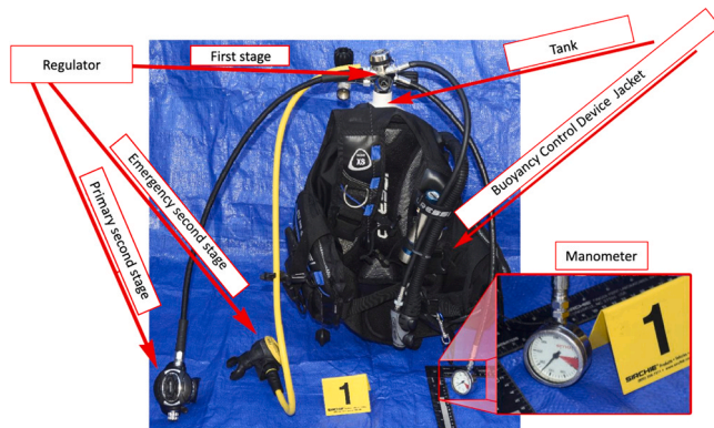
Fig. 2. Equipment in case#2 (SCUBA).
