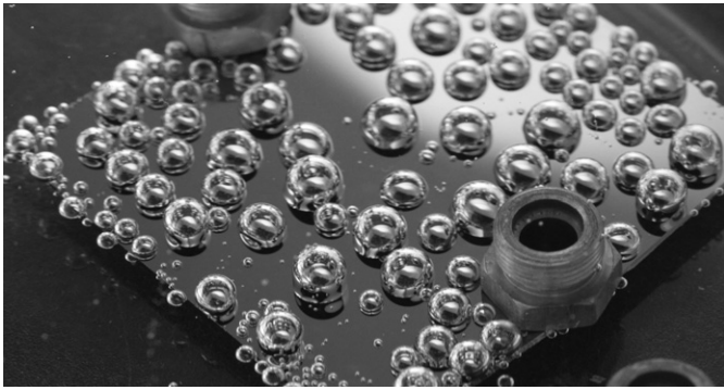
Fig. 2. Side view of a hydrophobic UW-I-wafer with brass weights photographed 1.5 h after decompression. At that time, a large number of bubbles floated to the water surface. Bubbles are spherical in shape, with reflections of other small bubbles and a mirror image from the smooth surface of the wafer.
