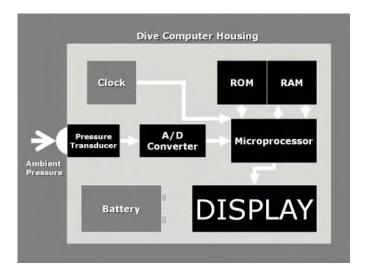
FIGURE 1. Dive computer schematic.
