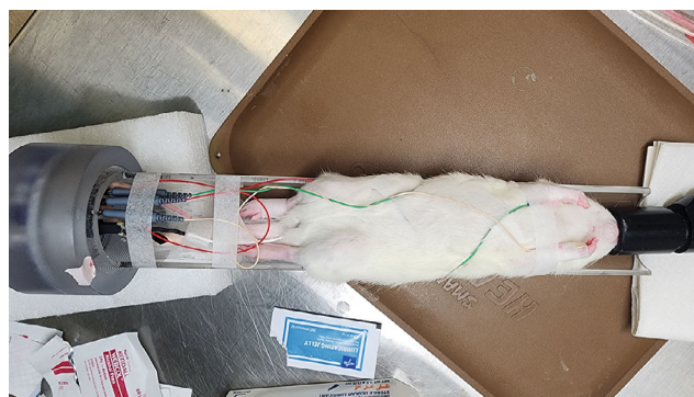
FIGURE 2 A rat is secured on the pressure chamber tray with electrocardiography wires arranged in an E-RESP configuration, which consists of a wire looped around its chest to generate induced voltage changes from respiratory movements in the presence of a magnetic field, and an inserted rectal temperature sensor.
