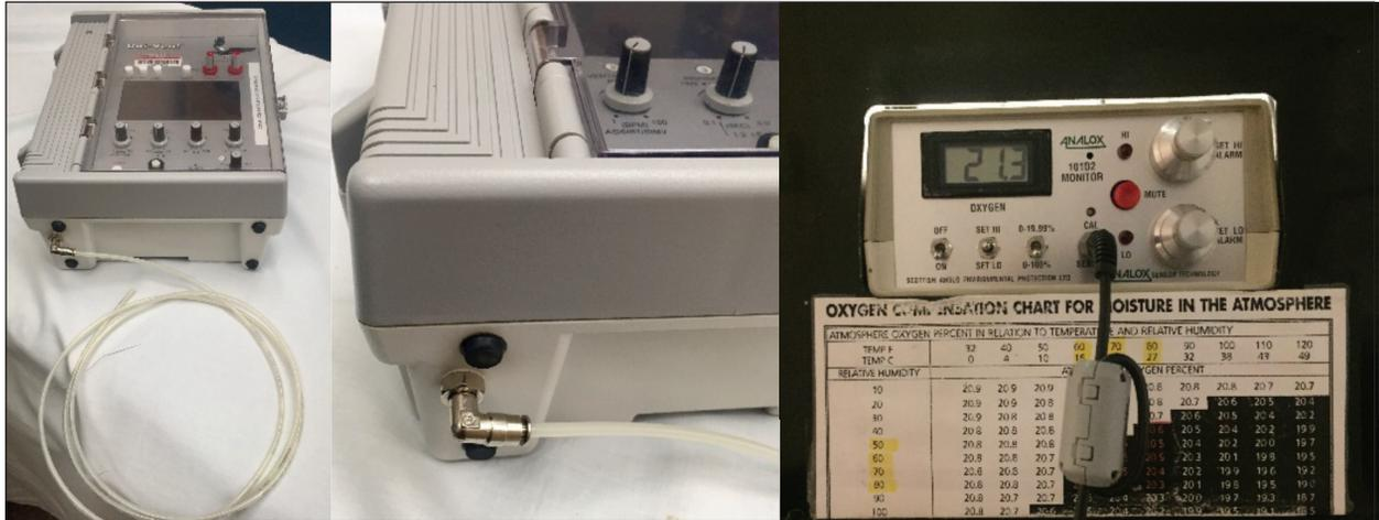
The sample port (with close-up view) drilled into the ventilator housing in order to sample the internal oxygen concentration using the Analex 101D2 monitor (bottom panel).
