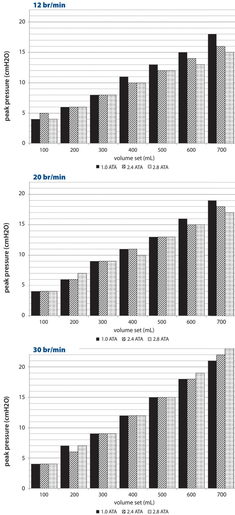
**Figure 6.** Peak pressures increased with faster respiratory rates and breath stacking in the higher set tidal volumes, especially at the 30br/min setting.
