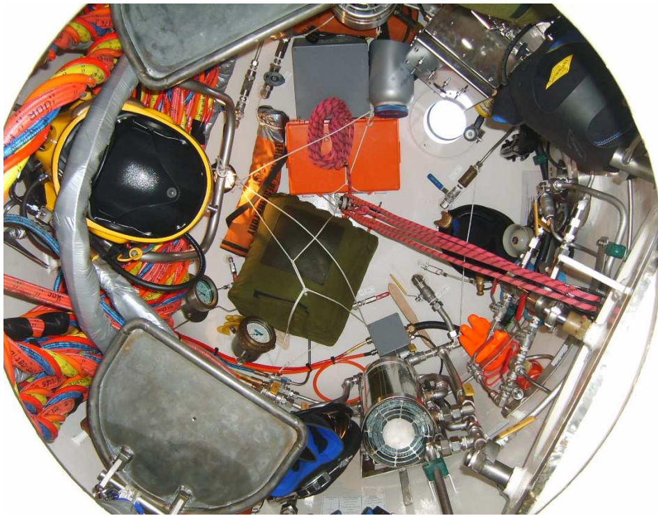
Fig. 5 Af-2 diving bell equipment seen from the entry (photo taken in 2016). We can see hoses and the bottom of the diving helmet used by the working diver.
