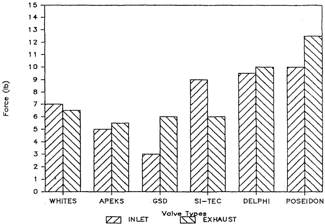
**Figure 11. Force required to activate valves (lbs.)**
