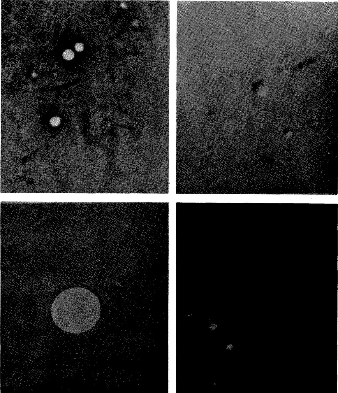
Near the center of the phase-contrast micrograph in the montage are two osculating nuclei, that is, two nuclei that are just barely touching and appear to be spherical in shape at the point of contact. Fig. 2 shows a similar binary nucleus photographed in distilled water with ordinary bright-field illumination (Yount *et al.*, 1984).
