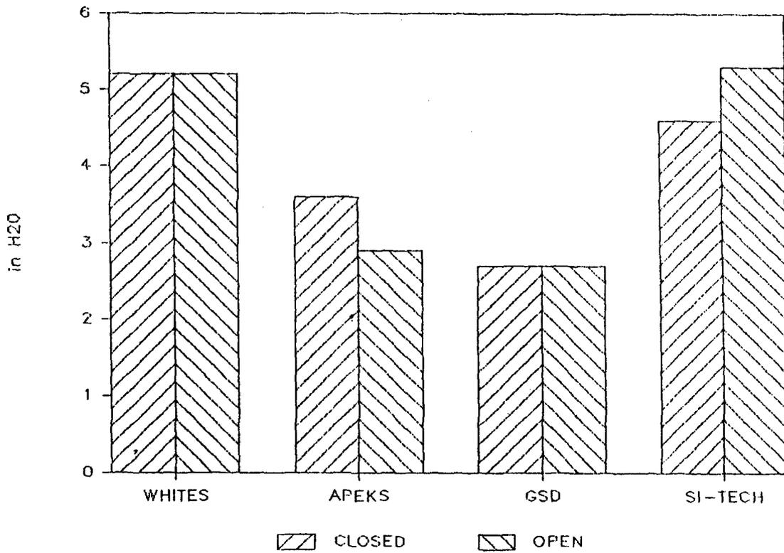
Figure 7. Pressure drop (inH<sub>2</sub>O), 5 cfm min/max opening pressure
