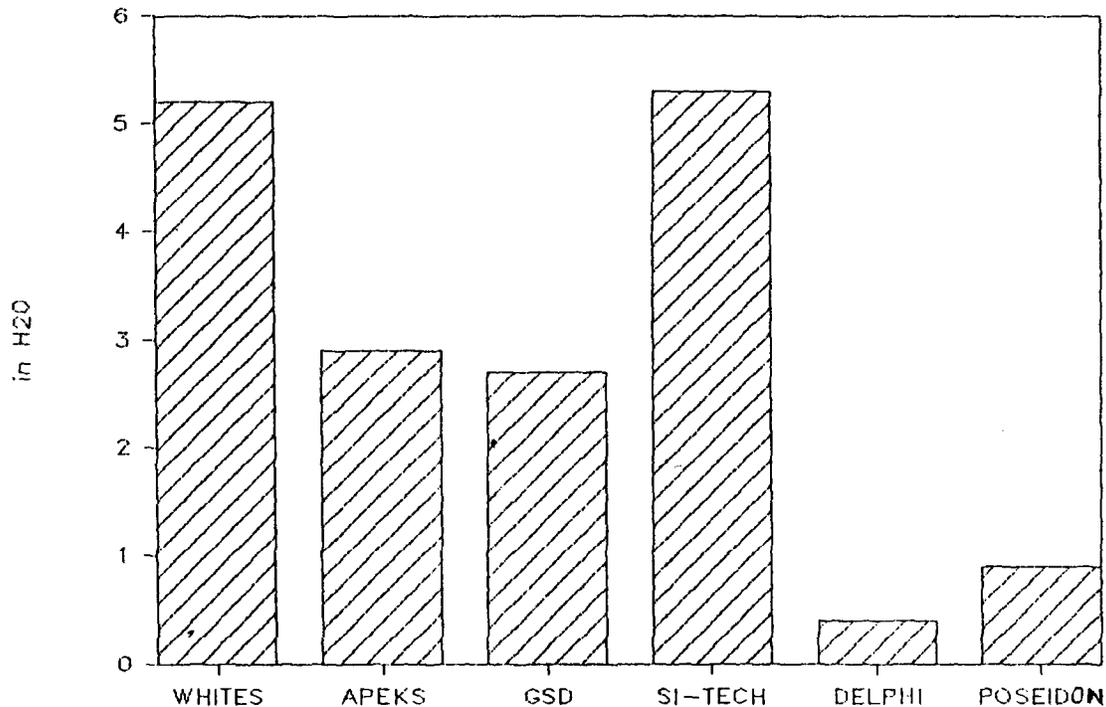
The force that is required to activate the valves is shown in figure 11. The two manual push to dump valves required the greatest force to activate. Although all the valves are grouped in a close range, I think we may consider that the MPD valves are near the upper limit for the force required to activate them.
