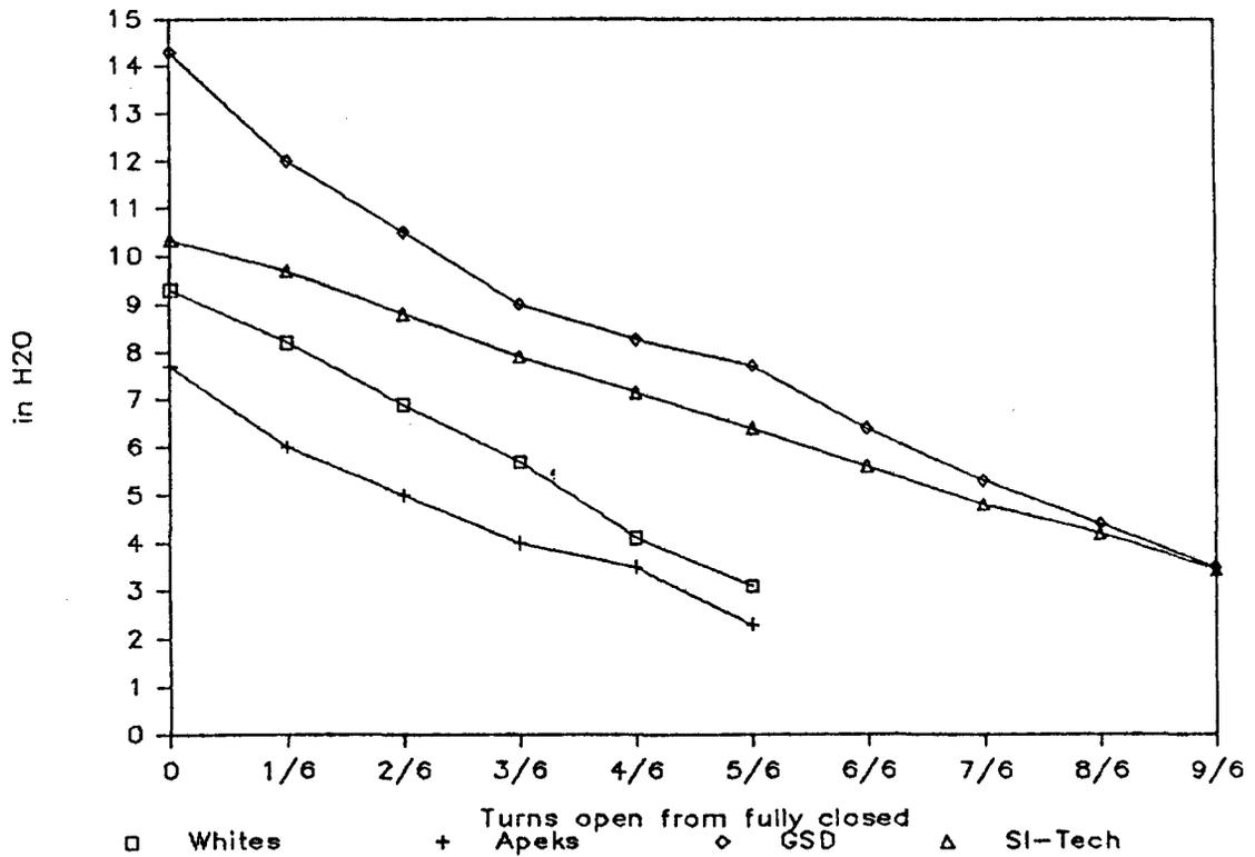
Figure 5. Pressure drop (inH<sub>2</sub>O) at 5 cfm
