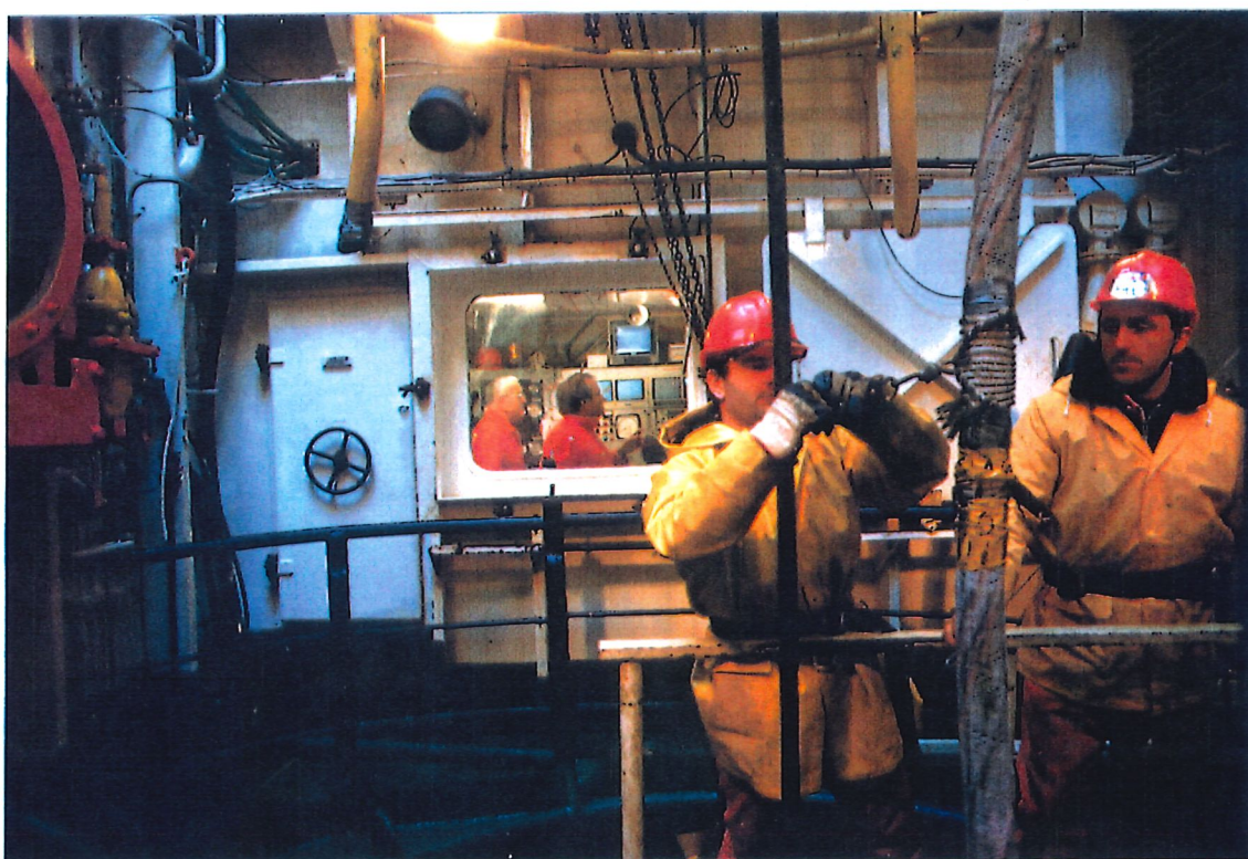
Moonpool - Descente tourelle Moonpool - Bell run down
