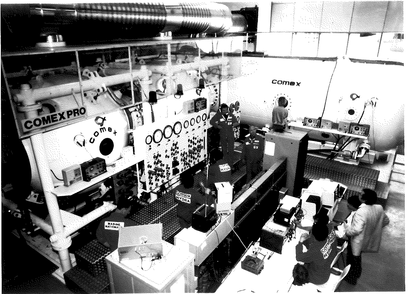
ENSEMBLE DE CAISSONS HYPERBARES ADAPTES AUX MELANGES HYDROGENES HYDROGEN MIXTURES HYPERBARIC CHAMBERS
