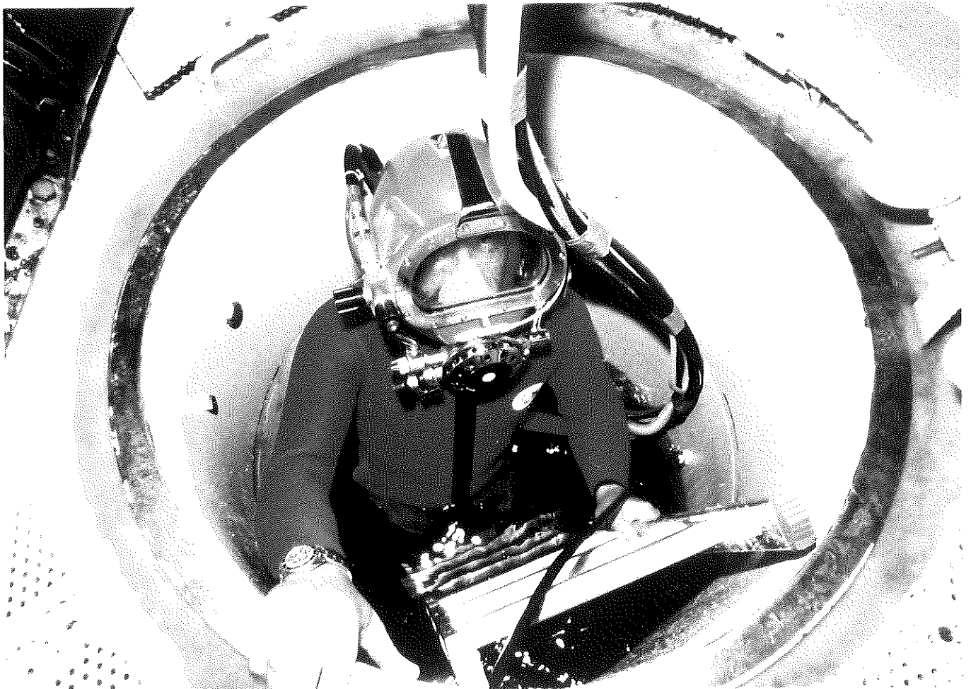
PLONGEUR EQUIPE DU CASQUE COMEX PRO T8 A 450 METRES SOUS MELANGE HYDROGENE DIVER EQUIPPED WITH COMEX PRO T8 HELMET AT 450 MSW UNDER HYDROGEN MIXTURES
