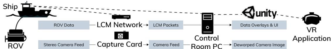
Figure 2: ROV-VR telemetry and camera data pipelines.
