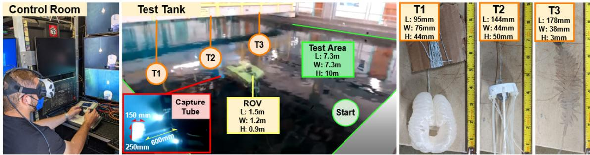
Figure 4: Experimental layout with measurements of the control room, test tank, and capture targets (T1-T3).
