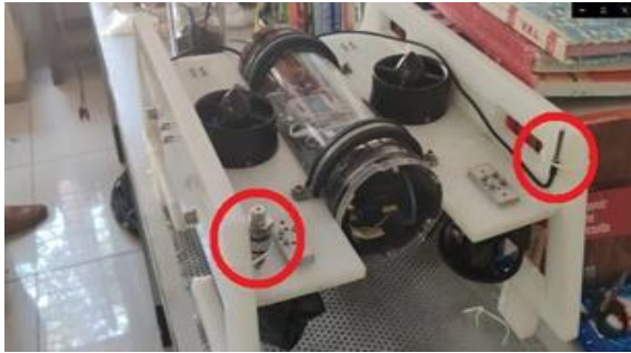
Figure 1. Representation of temperature and pressure sensor mounted on ORCA.
