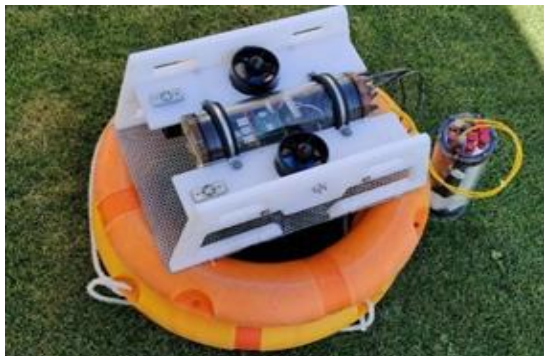
Figure 7(a) and 7(b): Fully fabricated ORCA with Integrated Navigation System
