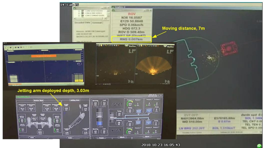
Figure 14. Verification of 3 m maximum trench depth.
