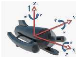
Figure 1. Underwater Vehicle Movement Design
