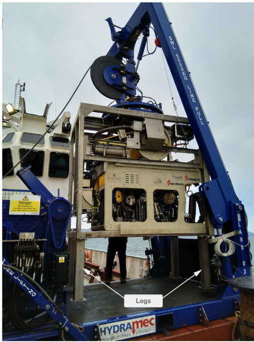
Fig. 4. The ROV within the TMS with four legs retrofitted for the static docking experiment prior to launch.
