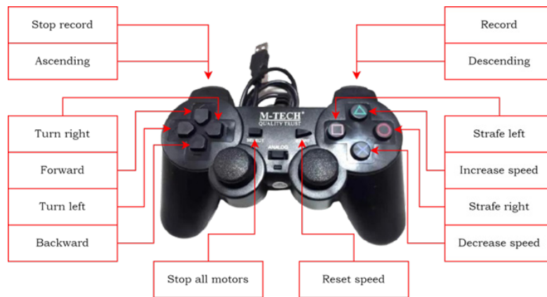
Figure 6. Layout of control buttons on the gamepad.
