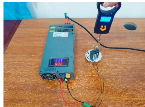
Fig.11 Experiment on electromagnetic adsorption force
