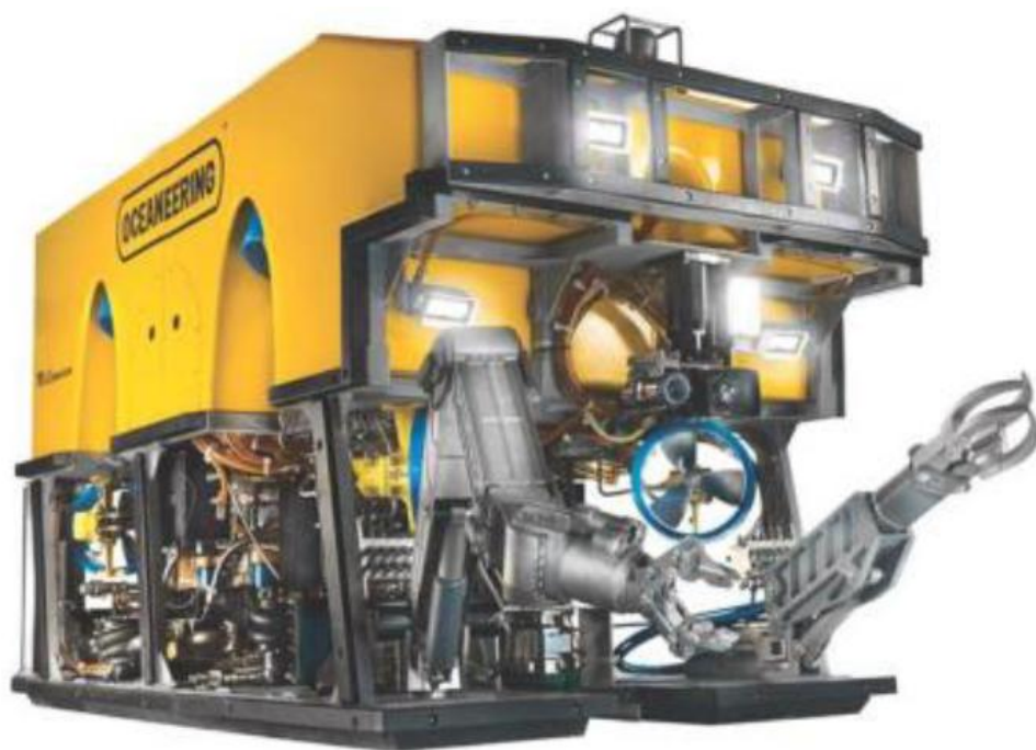
Figure 1. Work class ROV with an open box frame ROV design [12]
