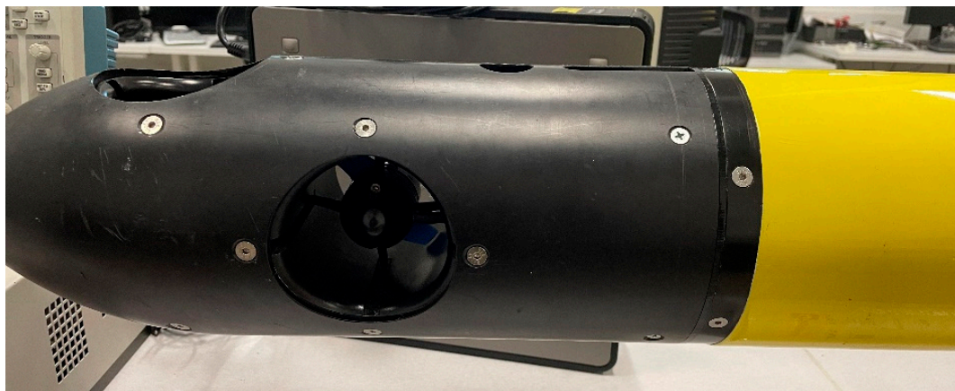
Figure 1. Side image of GRAALTech X300 AUV tail section showing a horizontal and vertical tunnel thruster pair.
