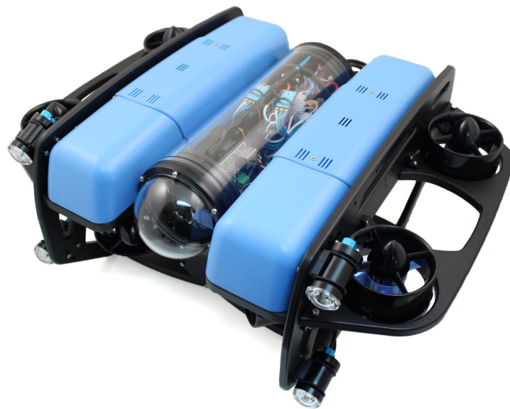
Figure 2. The BlueROV2 (BROV2) Heavy has eight thrusters; four are positioned vertically on the upper layer and four are positioned at symmetric angles on a lower plane.
