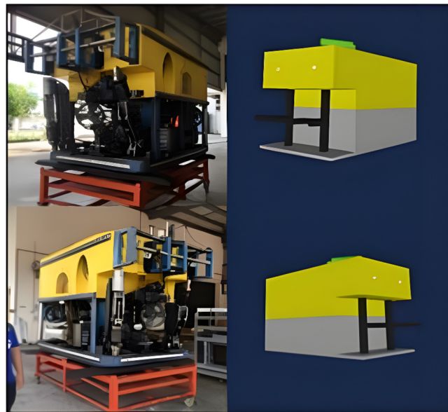
Figure 6. Top-left image: Front view of the actual working class remotely operated vehicle (ROV) used by Malaysian operators. Bottom-left image: Another angle of the actual ROV. Top-right image: The 3D model of the ROV as developed in our study, which replicates the front view of the actual ROV. Bottom-right image: An alternate perspective of the 3D model.
