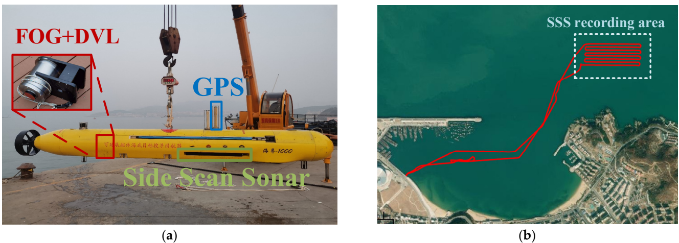
Figure 6. Physical experiment setup. (a) The sensors equipped on the AUV; (b) The experiment trajectory (the red line) and the SSS recording area.
