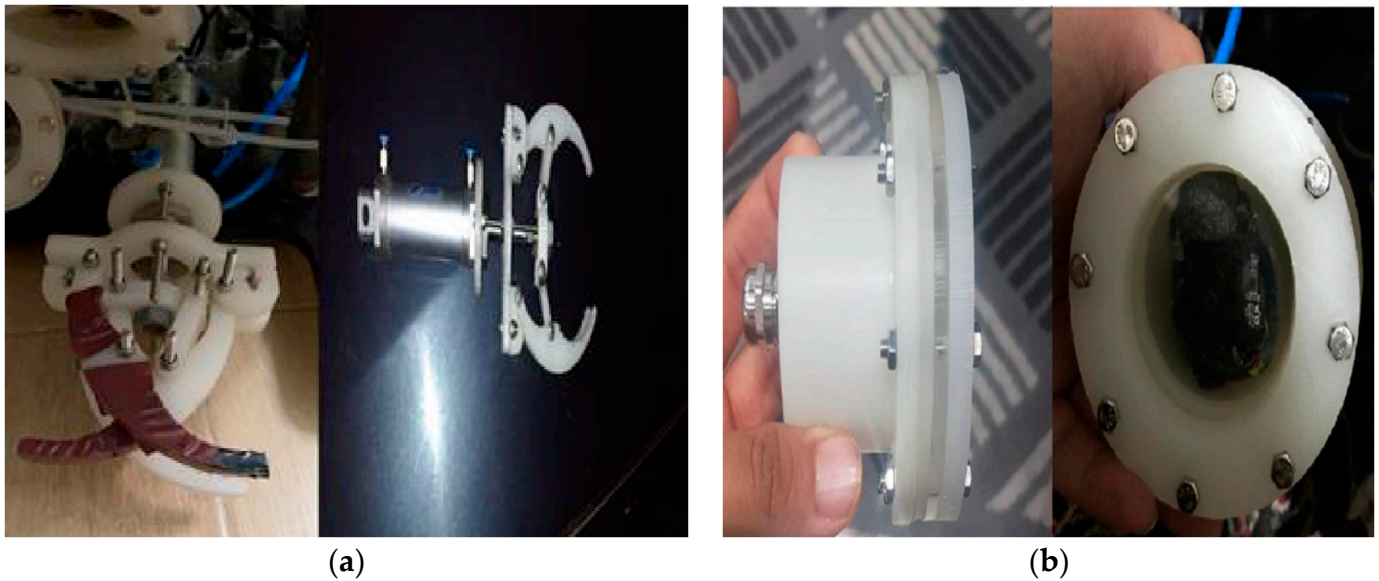
Figure 5. (a) Hydraulics gripper arm, (b) camera enclosure.
