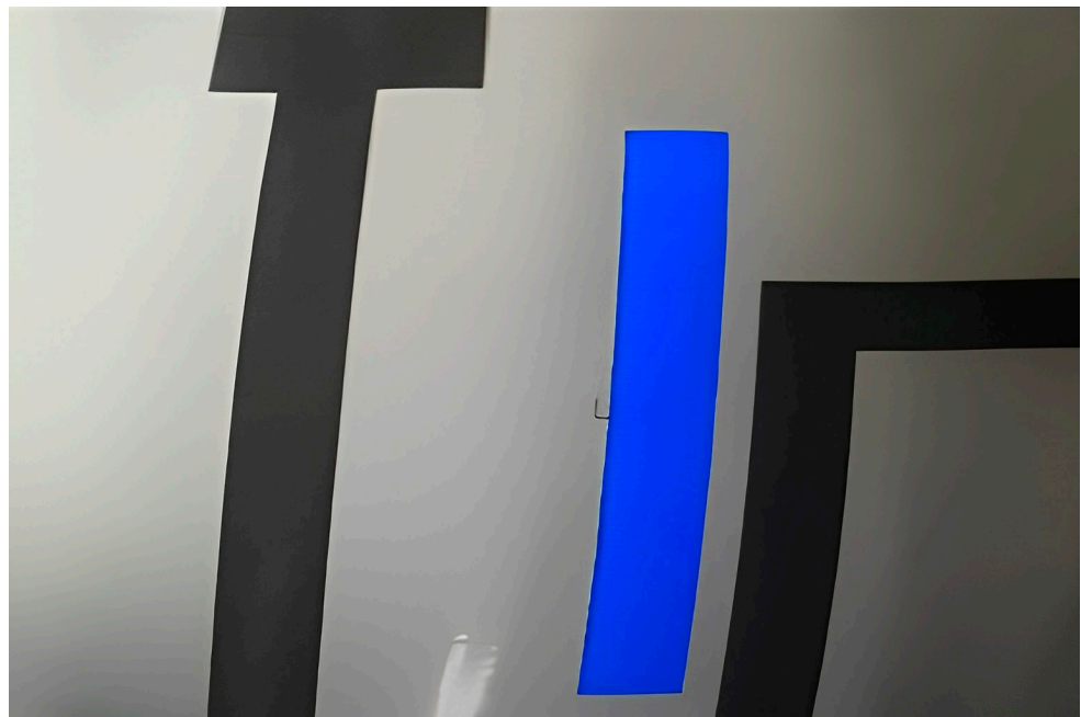
Figure 17. Crack length detection test. The blue line represents the crack.
