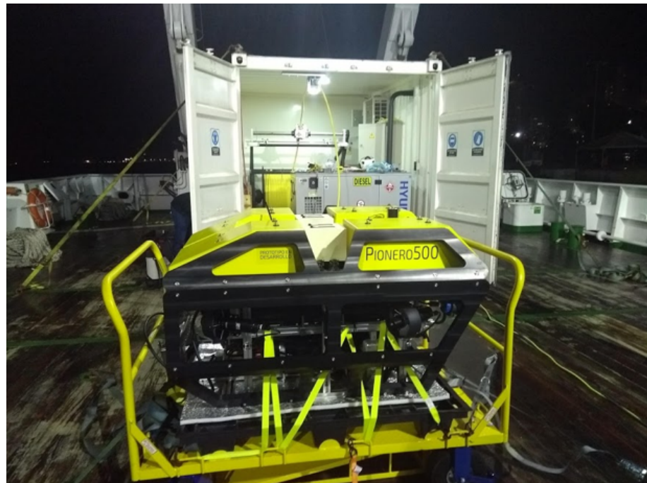
Figure 10. ROV Pionero500 (front) on board R/V ARC Roncador, with container with tether and backup power supply on the back.
