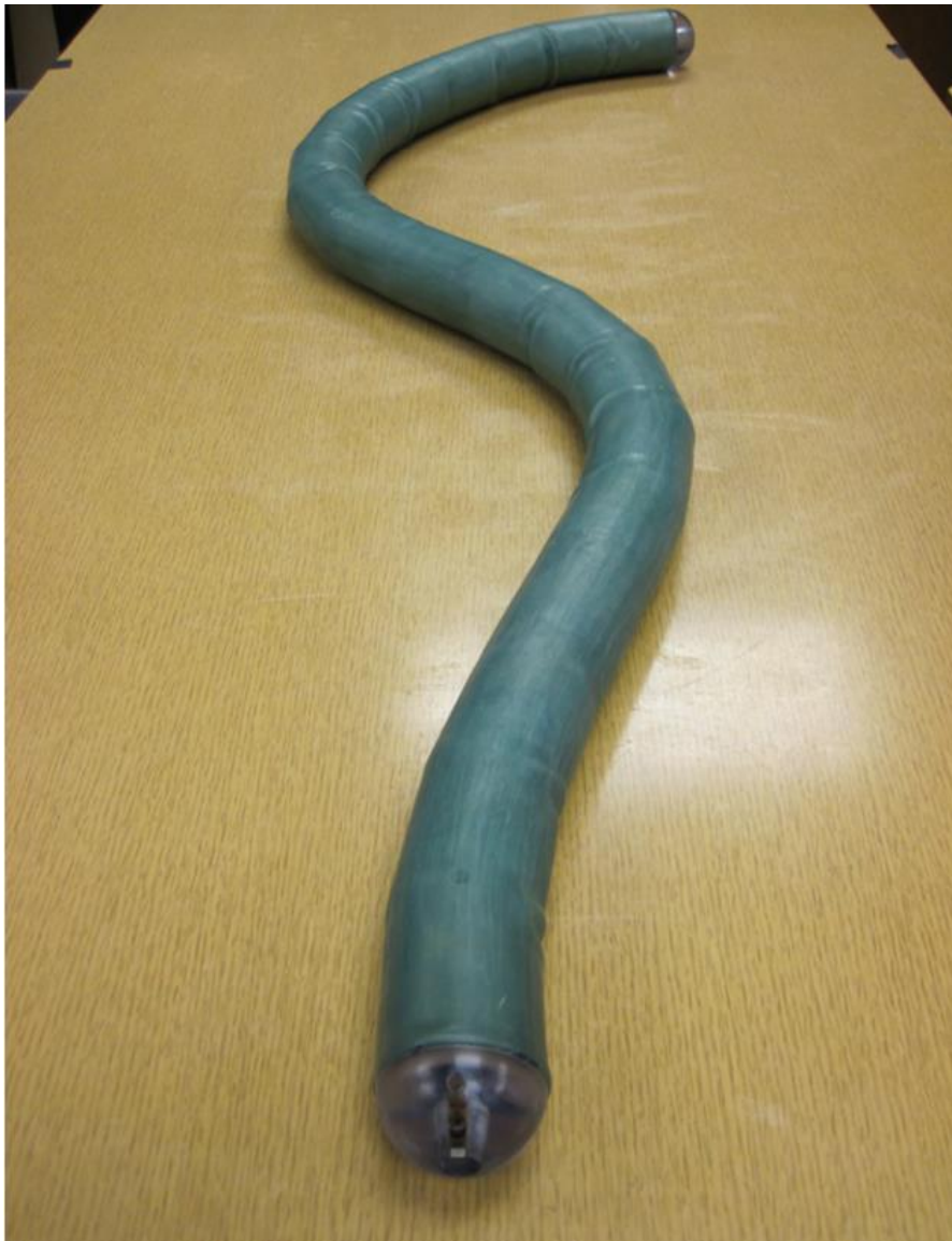
Fig. 4 NEELBOT-1.1 with the latex rubber skin. (Source: Potts (2015), Figure 3.2.1.3)
