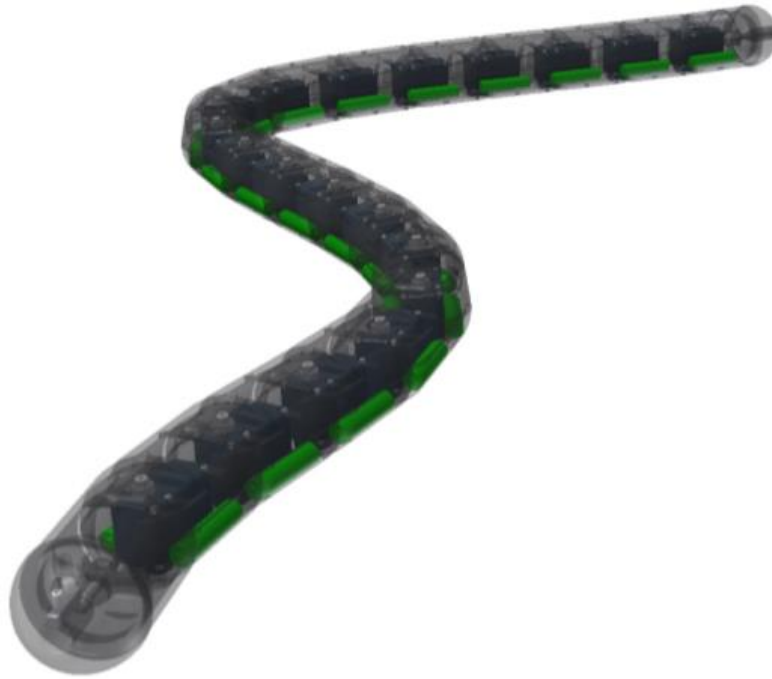
Fig. 5 Rendering of NEELBOT-1.1 showing off its sleek curves. The green cylinders are the AAA batteries with 2 per segment, and the dark blue boxes are the servo-actuators. (Source: Potts (2015), Figure 3.11)
