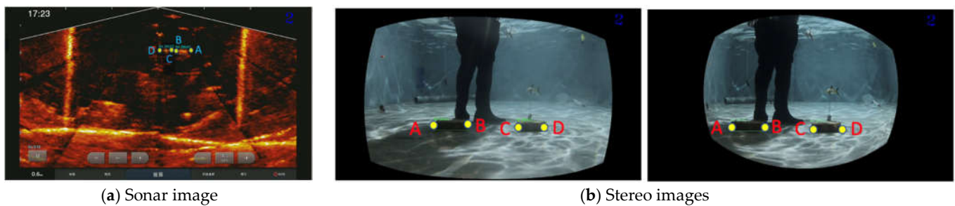
Figure 8. Brick detection and its corresponding four-point marks using YOLOv4 [55] in (a) sonar image and (b) stereo image pair.
