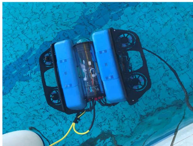
**Fig. 22** Tank test of BlueROV2 Heavy
