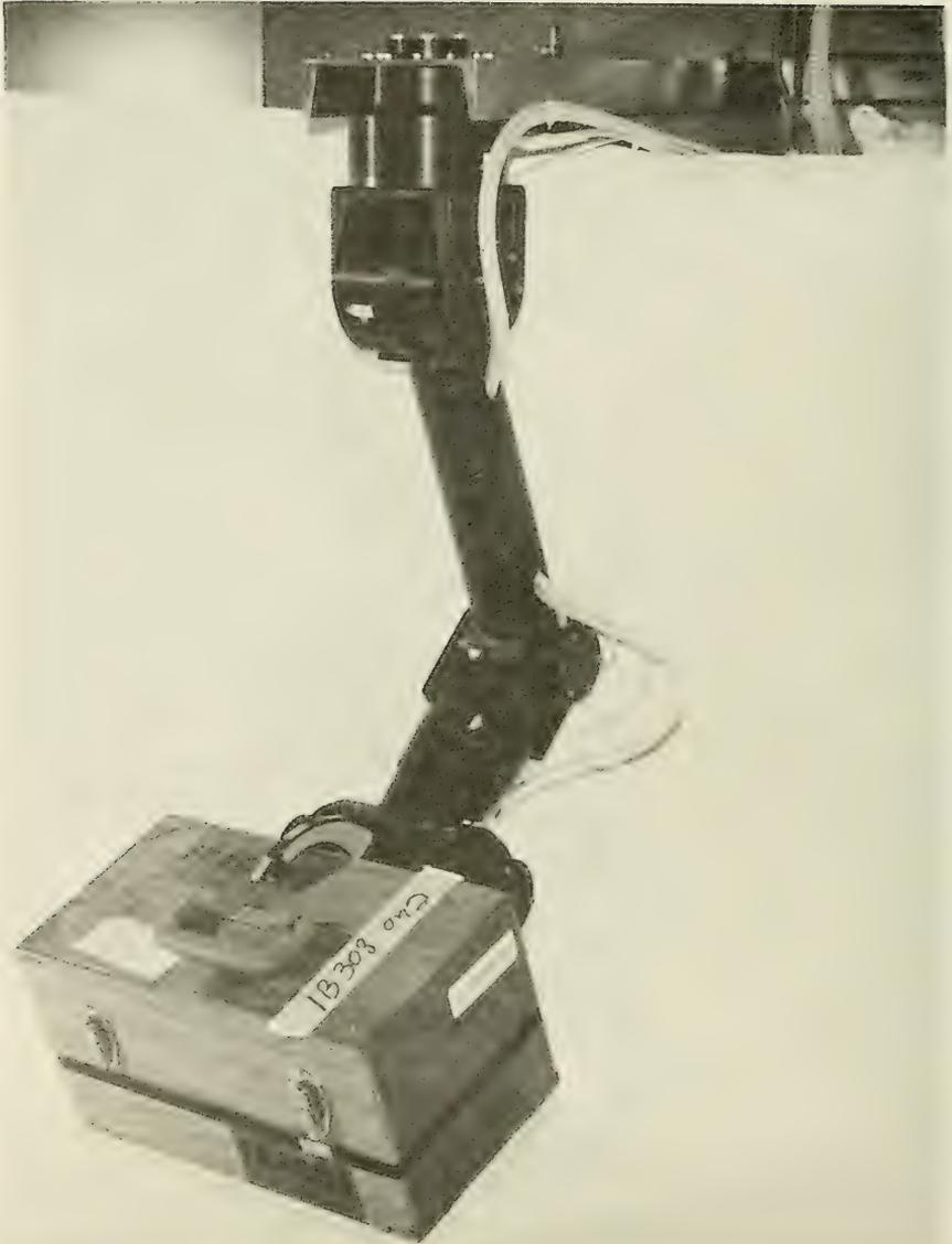
Figure 6. Manipulator shown grasping large object.
