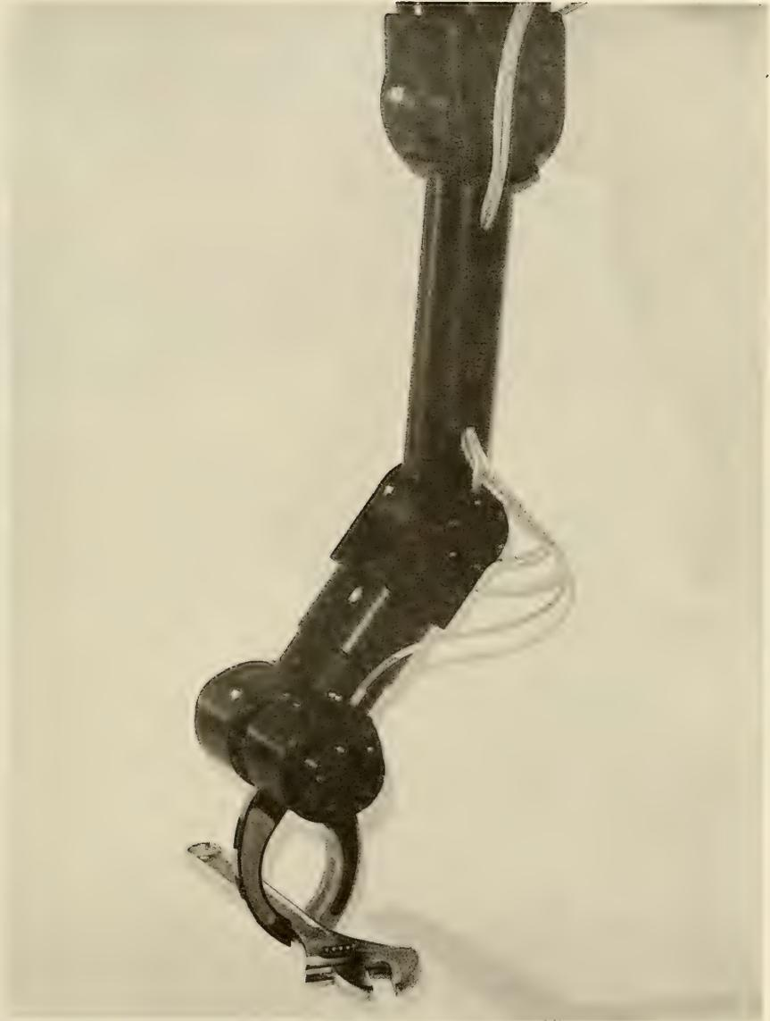
Figure 5. Manipulator shown grasping small object with "fingertips."
