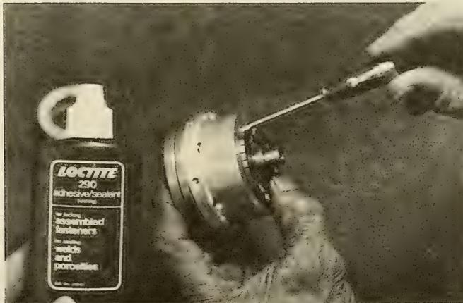
18. Secure the field with the four countersunk screws.
