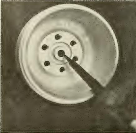
1. Clean all metal surfaces very thoroughly. Make sure that all deposits from previously used liquids such as cutting oils, masking paints, galvanic solutions, etc, are removed.
