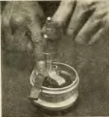
8. Put shaft into the ball bearing in the inner housing. The motor armature is in place when the distance from the inner housing surface to the surface of the rotor spacer is  $0.279 \pm 0.002$  inch.
