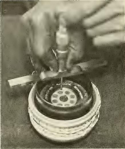
17. Put some drops of high-quality approved oil (MIL-L-6085A, MIL-L-8704A, MIL-L-644A) with a viscosity index of 70 into the bearing in the stator mount.
