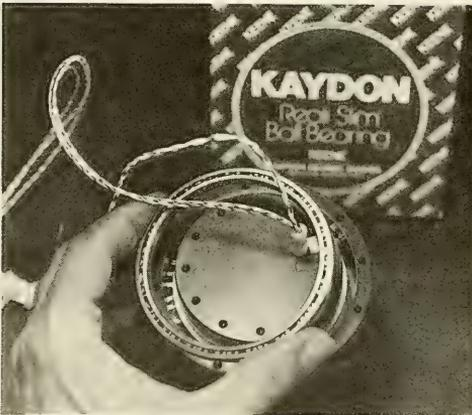
38. Press the Reali-Slim ball bearing (Kaydon bearing no KA040 XPO) into the housings so that the noninterrupted part of the bearing separator faces to the coil on the inner housing. Make sure not to transmit pressure or impact through the rolling elements of the bearing while pressing it into the housing.
