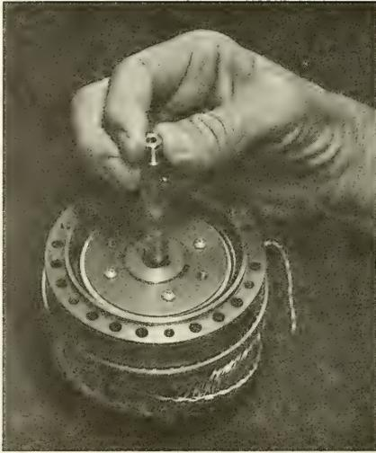
30. Put the key into the keyway of the shaft.
