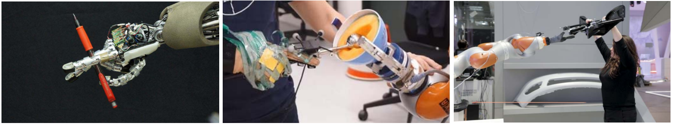
Fig. 6. Remaining challenges for robot manipulation. Dexterous movement of objects within the hand (left), manipulation of deformable objects (e.g., fruits and vegetables) (65) (middle), and manipulation of objects in collaboration with humans (right) present ongoing difficulties. [Photos: Learning Algorithms and Systems Laboratory, EPFL]
