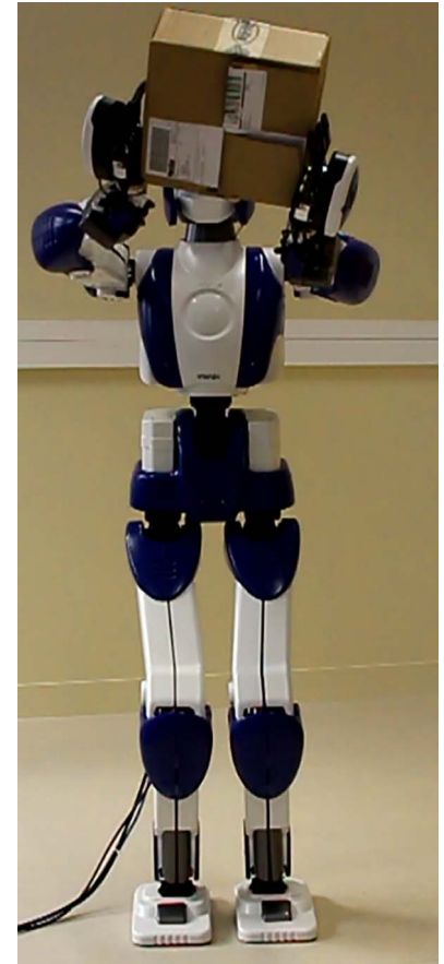
Fig. 7. Whole-body manipulation. Manipulation of a heavy object by a humanoid robot requires coordination of arms and body to maintain balance. [Reproduced from (74)]
