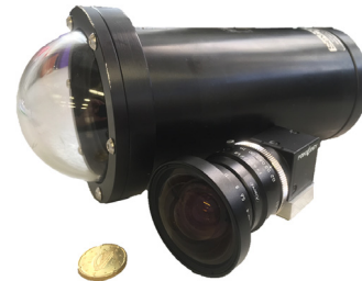
Fig. 7. Point Grey BlackFly camera with Kowa lens and a suitable subsea housing manufactured by Sexton.
