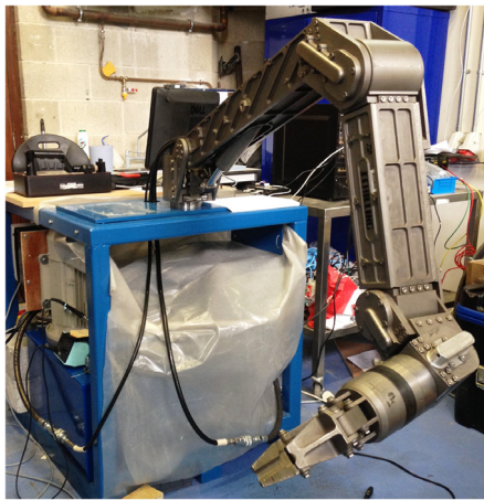
Fig. 5. Schilling Titan 2—hydraulic seven function subsea manipulator mounted on a lab test bench.
