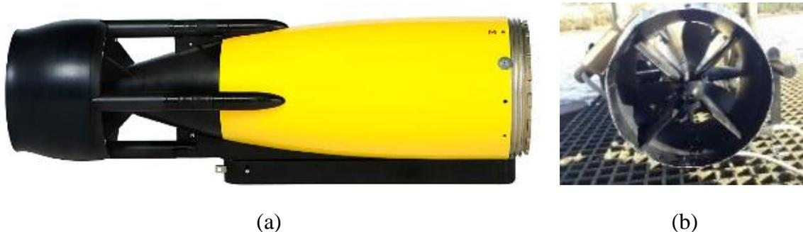
**Figure B.2 – Gavia Propulsion system. (a) Side View of the Propulsion Module. (b) The Control Surfaces in “X-wing” configuration**
