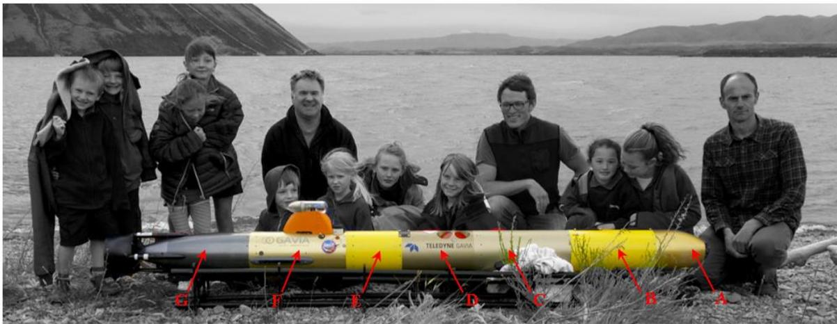
**Figure 5.1 – Omarama Primary School students inspecting the utilised *Gavia* AUV. Configuration of the vehicle – (A) Nose Cone Module, (B) Battery Module, (C) Geoswath Module, (D) ADCP/DVL Module, (E) INS Module, (F) Control Module and (G) Propulsion Module.**
