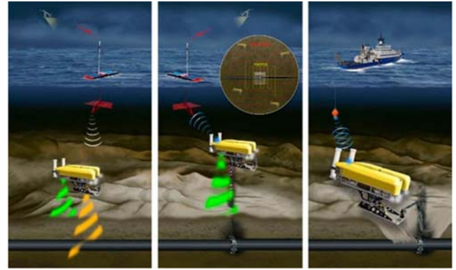
Fig. 9. Hybrid AUV inspection, monitoring, and intervention of seafloor and sub-seafloor pipelines concept.
