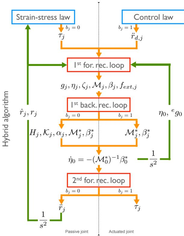
Fig. 2. Flow chart of the proposed hybrid algorithm.
