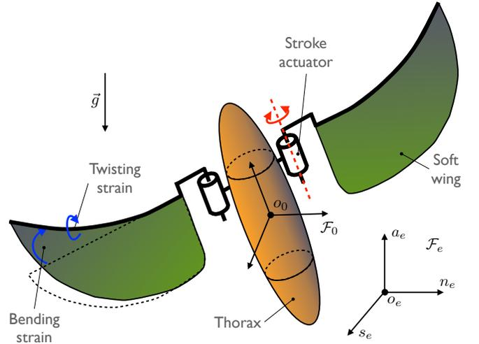
Fig. 3. Schematic view of the soft MAV.
