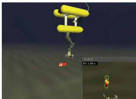
Fig. 4. Visual free-floating simulation intervention by using UWSim.
