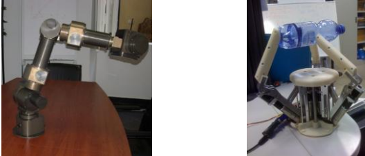
Fig. 5. (Left) the 7 DOF arm. (Right) the three-fingered dexterous hand.
